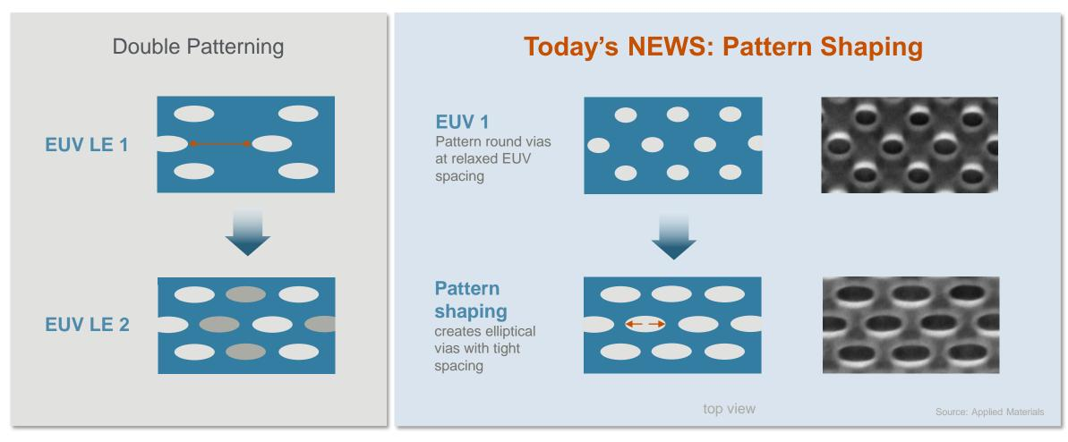
PPACt benefit: delivers high-density elliptical vias with only one EUV step, simplifying the patterning process flow – and optimizing chip power, performance, area and cost
