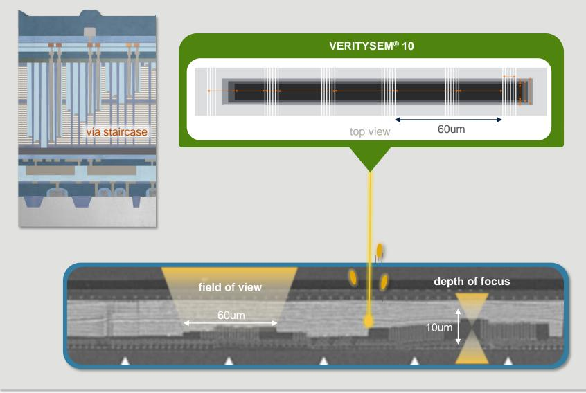
Staircase interconnect architectures increase contact density to reduce die area and cost. VeritySEM® 10 uses a large field of view with high depth of focus to measure the entire staircase structure with detailed step widths that help tune etch process recipes.
