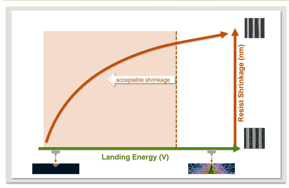
Landing energy: High eBeam energy increases interaction with the photoresist material, resulting in excess shrinkage and pattern distortion.
