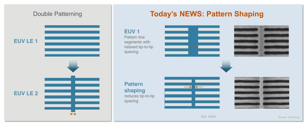
PPACt benefit: delivers the density of EUV double patterning with only one EUV step, simplifying the patterning process flow and optimizing chip area and cost
