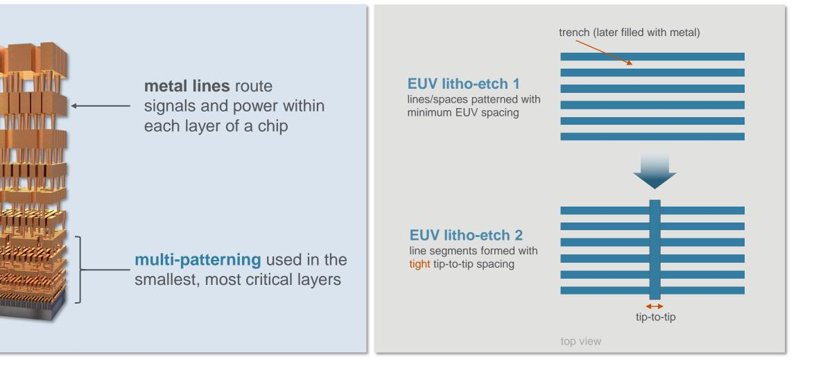
Tighter tip-to-tip spacing enables higher device density, which optimizes die area
