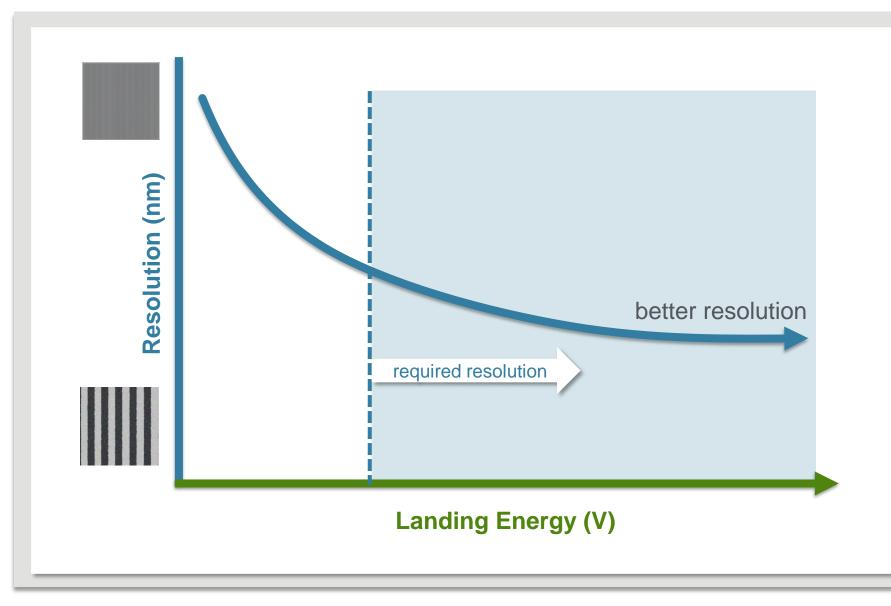
Landing energy: high energy is used to concentrate the electron beam on the target area and produce higher resolution images.
