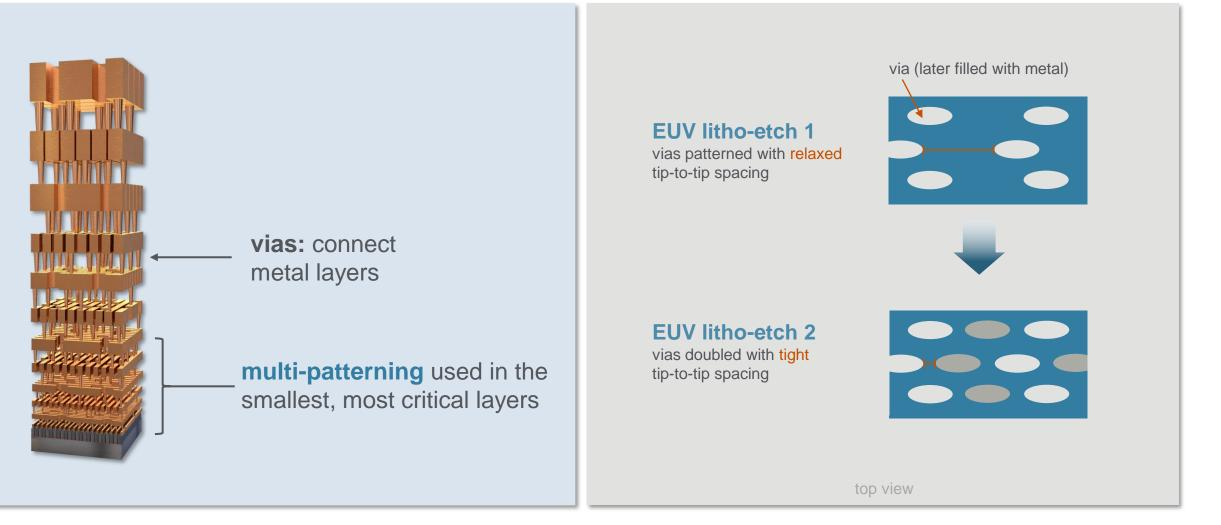
Elliptical vias provide larger electrical connection areas which optimize power, performance and yield Tighter tip-to-tip spacing increases via density which optimizes die area and cost
