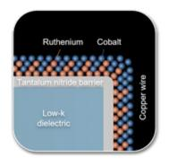
With the semiconductor industry's first use of ruthenium in high-volume production, Applied Materials' new binary metal combination of ruthenium and cobalt (RuCo) enables copper chip wiring to be scaled to the 2nm node and beyond and reduces electrical line resistance by as much as 25 percent.
