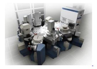
The joint lab features several of Applied Materials' 200mm and 300mm wafer processing systems, such as this Endura® system, and leverages CEA-Leti's world-class capabilities for evaluating performance of new materials and device validation.
