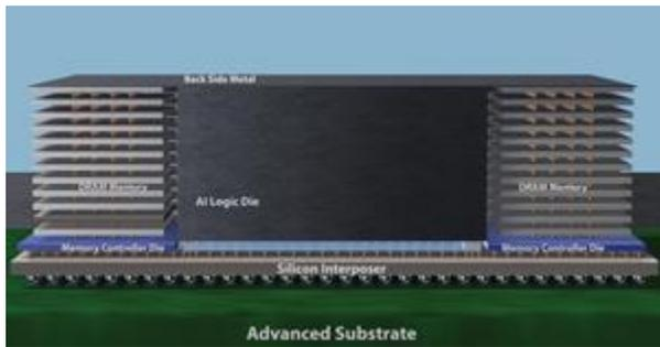
Heterogeneous integration brings new kinds of design and manufacturing flexibility to semiconductor and systems companies by allowing chips of various technologies, functions and sizes to be integrated in one package. Applied Materials is combining its leadership in process technology and large-area substrates along with ecosystem collaborations to accelerate the industry's heterogeneous design and integration roadmaps.
