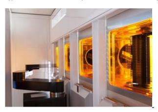
Applied Materials' new VIISta® 900 3D hot ion implant system injects and diffuses ions into 200mm and 150mm silicon carbide wafers, delivering a more than 40X reduction in resistivity compared to room temperature implant.
