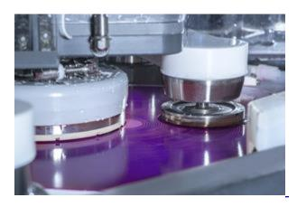
To help enable the silicon carbide chip industry's move to larger, 200mm wafers, Applied Materials introduced the Mirra® Durum™ CMP system. It produces uniform SiC wafers with the highest quality surfaces by integrating polishing, materials removal measurement, cleaning and drying in a single system.
