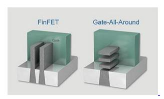
Gate-All-Around (GAA) transistors will be one of the chip industry's biggest design inflections since the introduction of FinFETs in 2010. Innovations in materials engineering provide GAA transistors with improvements in power and performance.
