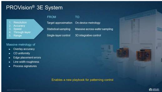
Relating back to the new patterning control playbook, PROvision 3E helps customers accelerate the transition: first, from target-based approximation to actual, on device metrology; second, from statistical sampling to massive across-wafer sampling; and third, from single-layer control to 3D integrative control.
