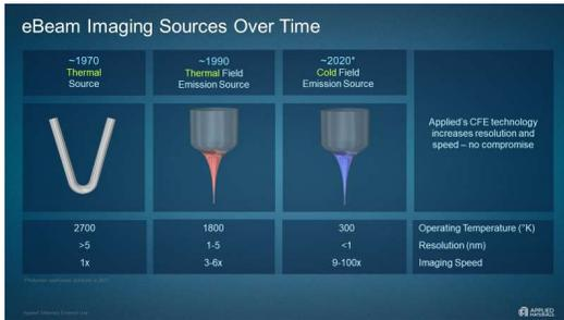
The technology is called “cold field emission” or CFE. It has two simultaneous benefits. First, it enables sub-nanometer resolution. Second, we can produce two to five times more electrons at the same resolution as conventional eBeam technologies.
