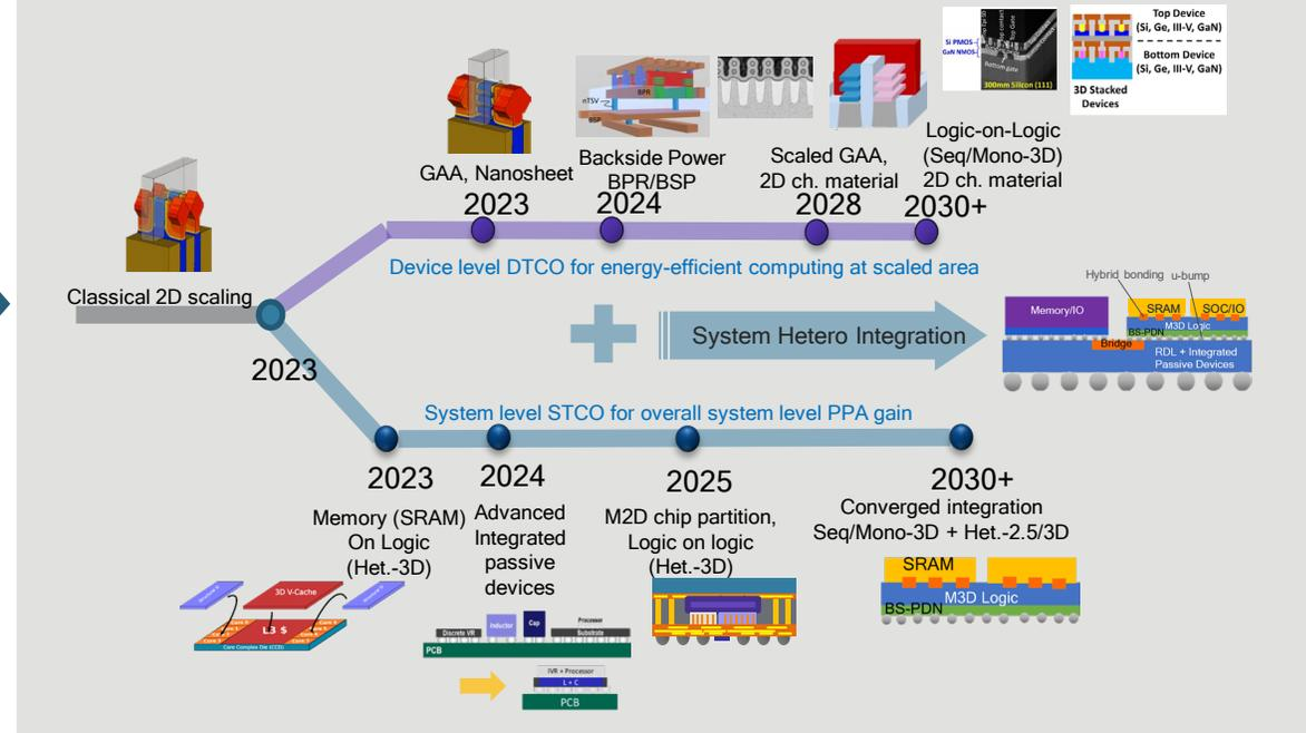
Advanced packaging enables high density interconnects with larger die complexes from multiple process nodes
